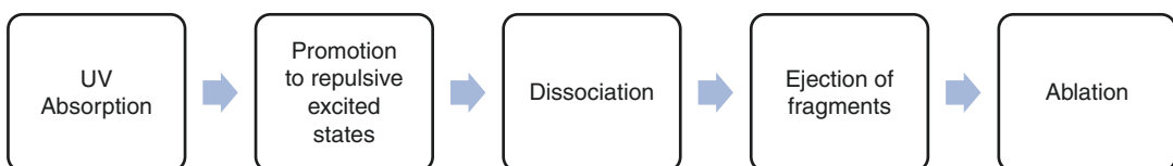
Fig. 3.5 Summary of the principle of photoablation
