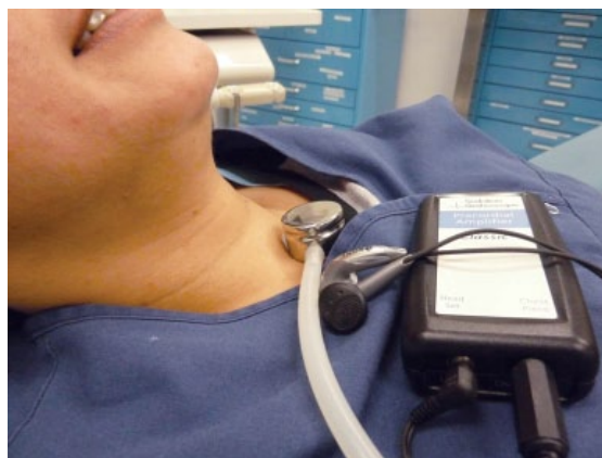
Figure 6.3 An amplified, electronic pretracheal stethoscope to monitor breath-to-breath respirations in a sedated patient. Photos (Capnography, Pulse Oximetry, Pre-tracheal stethoscope).
