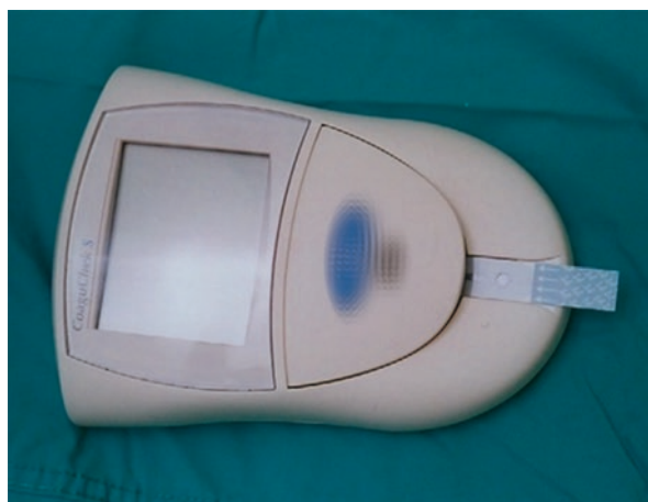
Fig. 10.5 The INR can be measured at the chair side by portable machines that require only a finger-prick blood sample
